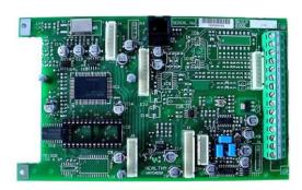
Flexible digital signal conditioning amplifier for multiple or single load cell applications, offering very easy one-pass calibration and fast set-up
