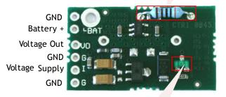
LED lights when supply voltage applied
