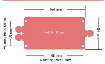
IP67 ABS field case fitted with 3 M16 cable glands Cable diameter: 4mm (0.16") to 7mm (0.27")
