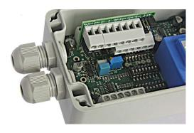
Screw the SGABCM Module into the normal load cell connector J2
