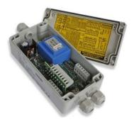
SGA with a retro fitted bridge completion module pcb.
