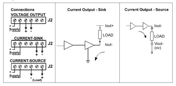
In **'Sink'** mode the +ve end of the load is connected to the internal +15V supply on the LVDT and the -ve end is connected to the LVDT output. The current through the load is 'sunk' by the LVDT towards ground (0V). N.B. In this mode neither connection to the output load is electrically common to the load cell. Select this option by fitting the two jumpers in the positions next to the span trimmer (See Output Current Mode Settings - Jumpers JP1 & JP2)
