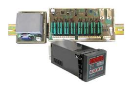
The DIN rail mounted remote relay units offer an increased number of set points over that provided by a standard ADP15 indicator / controller: this allows for multi action operations
